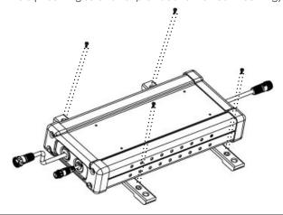
7. Connect the lamp to the power supply through the 3-pin snap connectors. Additional 3 and 6 foot extension cords are optional equipment. Connect the AC adapter cord to the input side of the power supply (3-pin threaded). \*Optional dimming function can be controlled through 0 - 10V dimming cord accessory.
